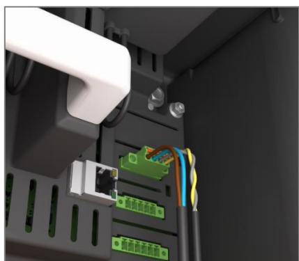
Connect Communication Wiring in Backup Gateway
